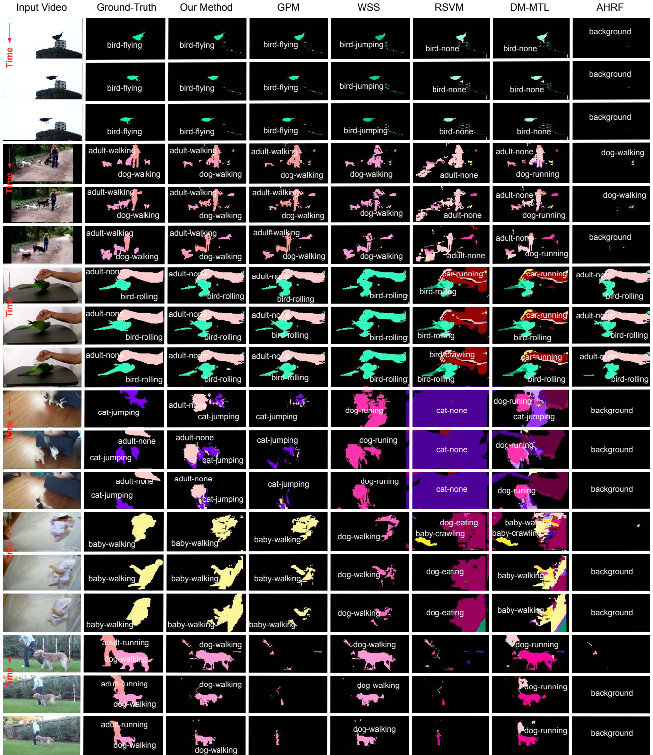
Figure 4. Qualitative results shown in sampled frames for several video sequences from the A2D dataset. Columns from left to right are input video, ground-truth, our method, GPM [58], WSS [54], RSVM [23], DM-MTL [22] and AHRF [28] respectively. Our method is able to generate correct actor-action segmentation expect for cat-jumping and adult-running in these examples.
