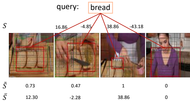
Figure 4. Example to show how the contextual similarity works with numerical demos. The grounded boxes are localized by our full model and box color is defined the same as Fig. 2.
