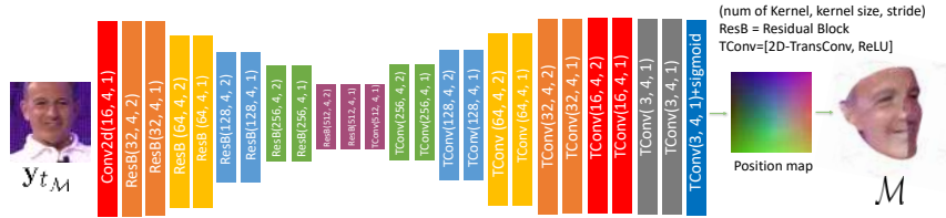
Fig. 3. The details of the unprojector. We use the method proposed in [4] as the unprojector.
